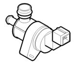
The evaporative emission system (EVAP) valve is used to open and close the connection between the EVAP canister and the intake manifold. The valve controls the flow of hydro-carbons (fuel vapor) from the EVAP canister to the engine intake manifold using the vacuum in the
