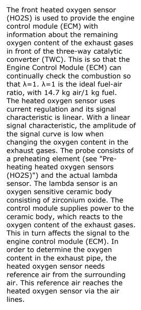
Caution! The wiring for the heated oxygen sensors (HO2S) must not be trapped or damaged in any way. The connectors for the heated oxygen sensors (HO2S) must not be greased under any circumstances. The oil in the grease would disrupt the reference air and the function of the heated oxygen sensors (HO2S).
