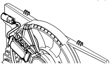
The engine cooling fan (FC) cools the coolant, engine compartment and the condenser when the air conditioning (A/C) compressor is running.
