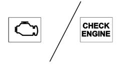
The emissions warning lamp in the Driver Information Module (DIM) has a warning symbol. This warning symbol varies
