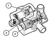
The function of the leak diagnostic unit is to pressurize the fuel tank system during leak diagnostics and to open the fuel tank system to the surrounding air during evaporative emissions control.
